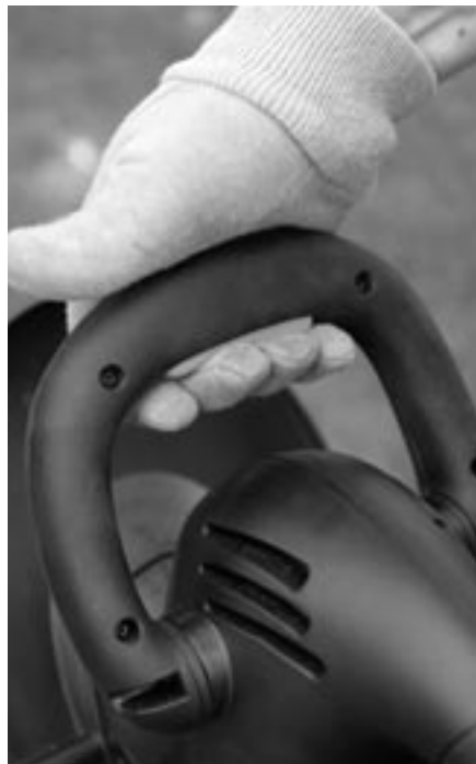
Figure 3-6: Positioning hand on front handle
